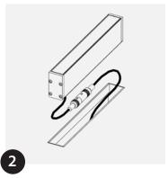
Make power connection to suit IP requirements of installation location. Insert MOMO-F.
